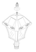
7. Assemble pole by screwing the four pieces together.
